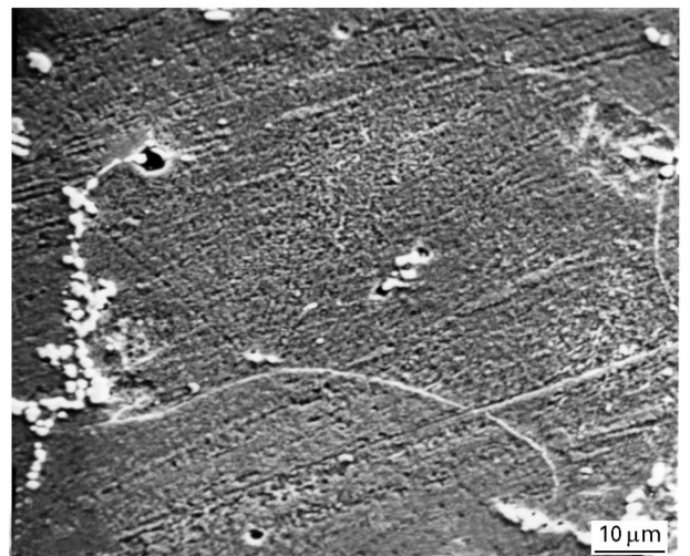
Figure 6 SEM image of the surface of the specimen implanted with a 1.5 \times 10^{17} \text{Si}^+ \text{cm}^{-2} dose after the anodic polarization.
